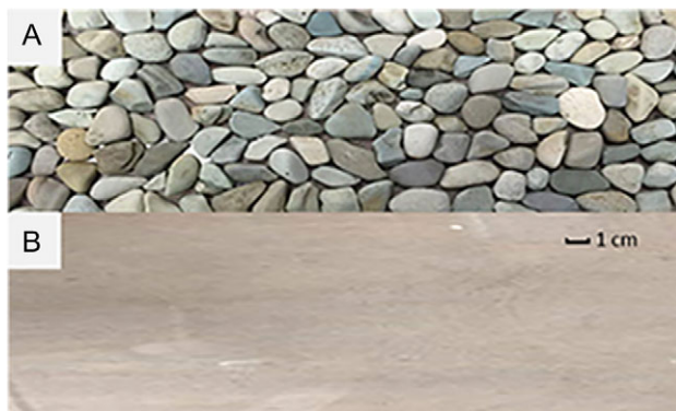
Figure 1: Substrates used in the swimming trials: (A) roughened substrate with fixed river stones and (B) smooth acrylic panel; River stones varied in shape and size but the majority were \sim 3 \times 2 \times 1 cm; l \times w \times h ; River stone length equated to 0.3 BL and 0.5 BL for purple-spotted gudgeon ( Mo. adspersa ) and crimson-spotted rainbowfish ( Me. duboulayi ), respectively.
